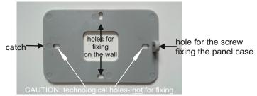
When the back cover of the control panel has been installed as shown, the panel (already activated and paired) should be fixed to the back cover using the latch on the left hand side. After the panel has been put in place, tie up the screw on the side wall of the panel's case.
